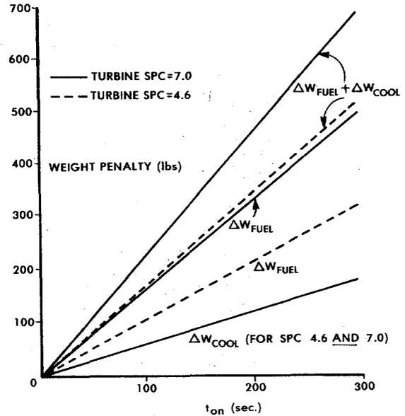
FIGURE 4 System Weight Penalties vs. Run Time
