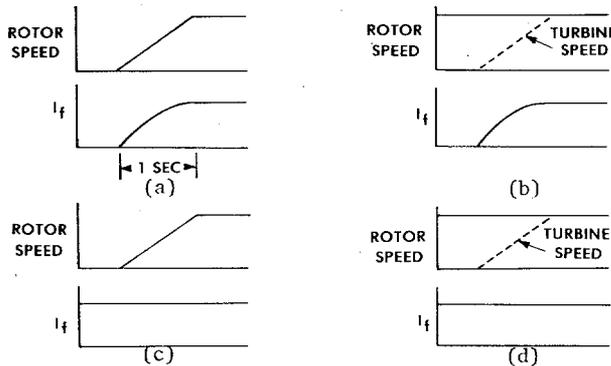
FIGURE 3 Possible Rapid Start-Up Methods
