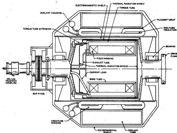
FIGURE 2 Advanced 20 MW Superconducting Generator (General Electric Co.)
