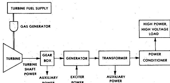
FIGURE 1 Generalized High Power, Airborne System
