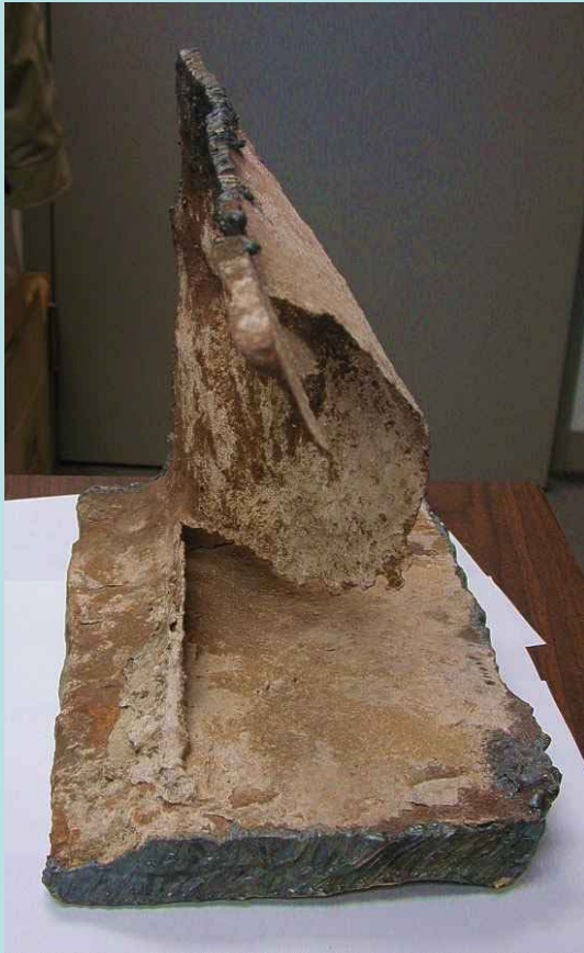
Column Section Showing Region with Severe Thinning
