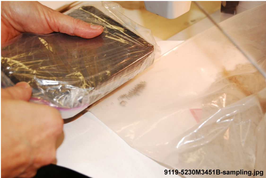
Figure 5. An example of separating particles with a magnet. Sample M3451 – Ann St.
