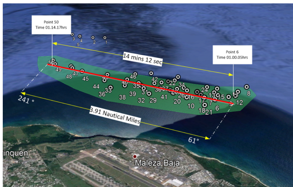
The Radar returns drift over time
