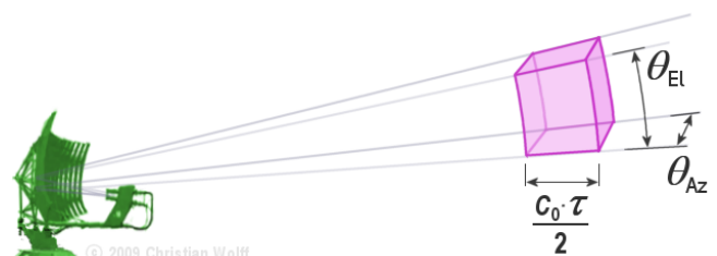
Figure 16: The resolution cell
