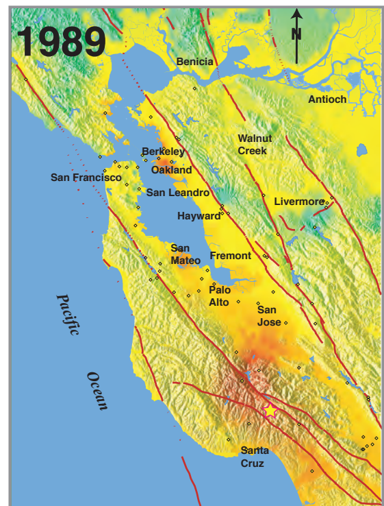
A ShakeMap showing the inferred intensity of ground shaking in the 1868 earthquake (MMI, or Modified Mercalli Intensity), compared to a ShakeMap for the 1989 magnitude 6.9 Loma Prieta earthquake. Red lines are earthquake faults; black line shows the portion of the Hayward Fault that ruptured in 1868; yellow star marks the epicenter of the 1989 quake. Diamonds show locations of damage reports (1868) and of seismic recordings (1989).
