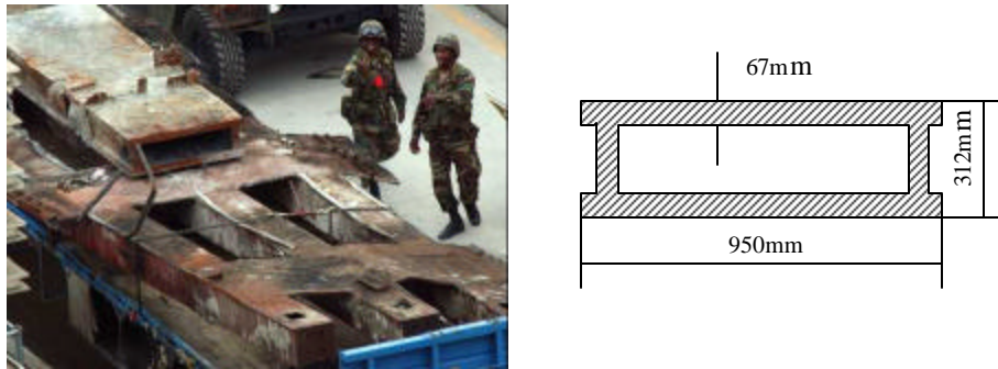
Figure 13. Relative size of core column compared to the exterior column. We have estimated the geometry of the core column from this photograph.
