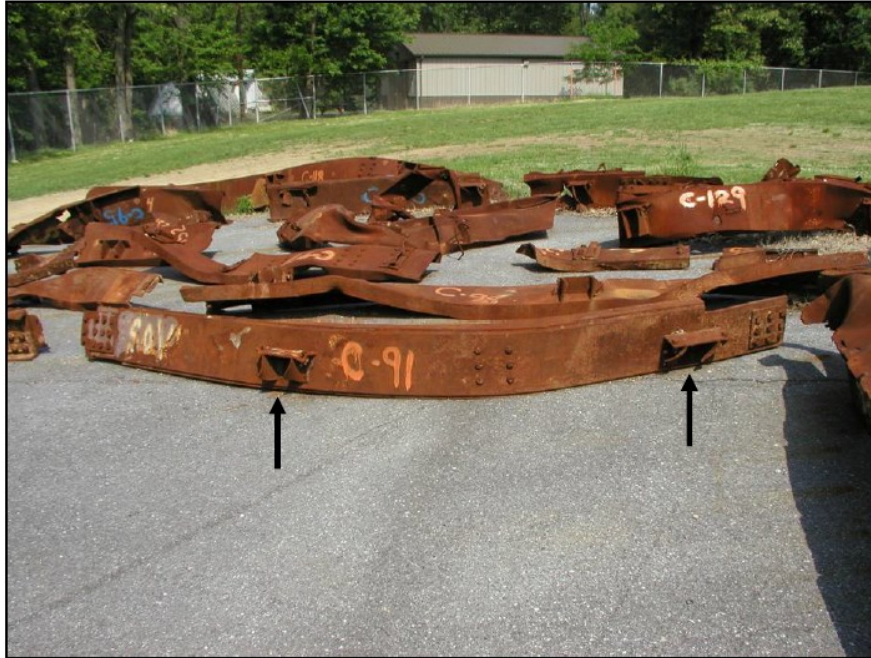
Figure 4-6. Example of a recovered core channel. Arrows indicate seats used to attach the floor trusses to the channel (core columns).
