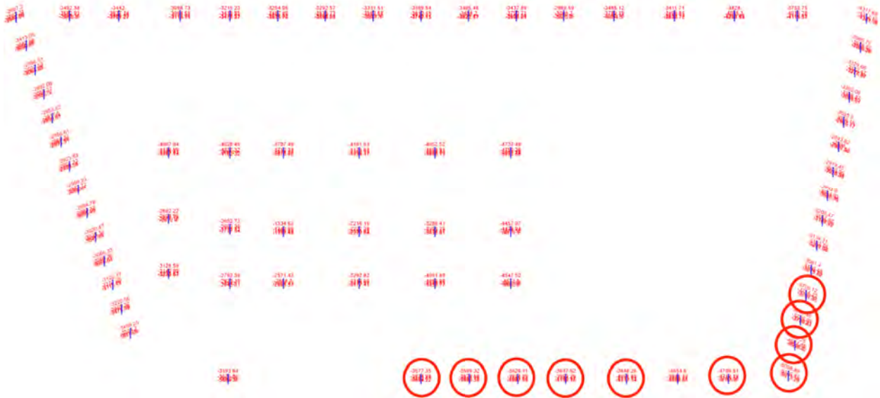
Figure 4.10: Linear static analysis results show that the failure of Columns 76 to 81 overloads 10 exterior columns (circled in red) around the southeast corner, but not the next row of core columns to the west (not circled in red).
