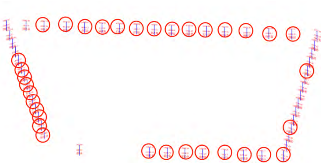
Figure 4.17: Linear static analysis results show that the simultaneous failure of all core columns leads to the failure of most exterior columns, causing the building to tip to the southwest. Only columns at the northwest corner and eastern side are not overloaded.
