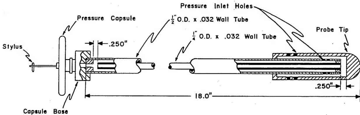
Figure 3.17 Details of pressure probe.
