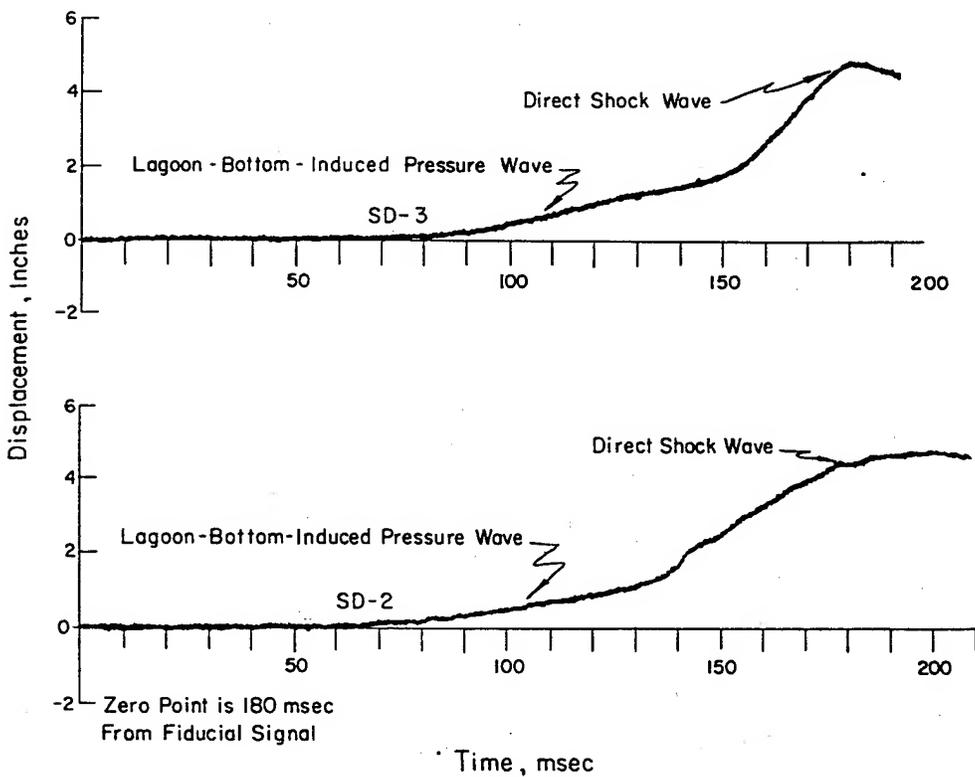
Figure 3.43 Vertical displacements on EC-2, Shot Umbrella.
