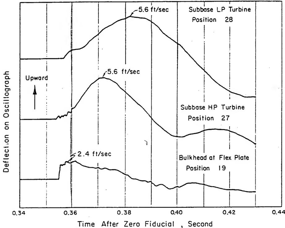
Figure 3.51 Vertical velocities of turbine foundation and subbases in USS Fullam (DD-474), for direct shock wave from Shot Umbrella.
