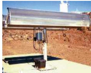
NASA/Boeing Company 1.3 kW CPV System (First kW-Scale CPV System Ever Installed Using Multi-Junction Cells)
