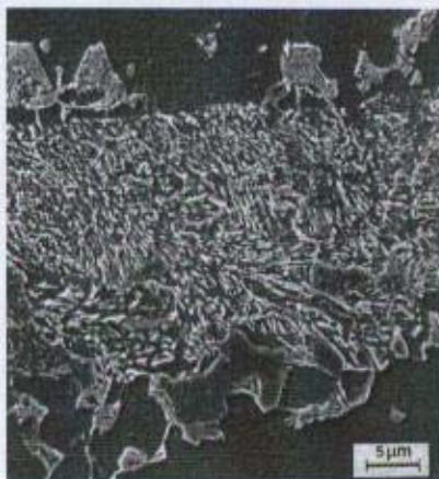
FIGURE 5 (left) SEM view of the start of spheroidization of lamellar cementite in the A36 steel beam (nital etch). FIGURE 6 (right) Recrystallization of ferrite in areas where the pearlite has been partially dissolved (nital etch).
