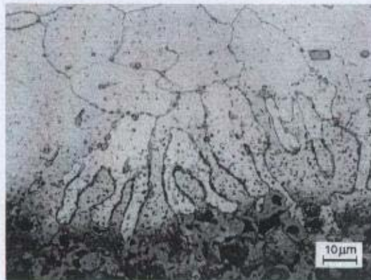
FIGURE 12 Example of grain-boundary decoration by the eutectic attack in the HSLA column material (nital etch).
