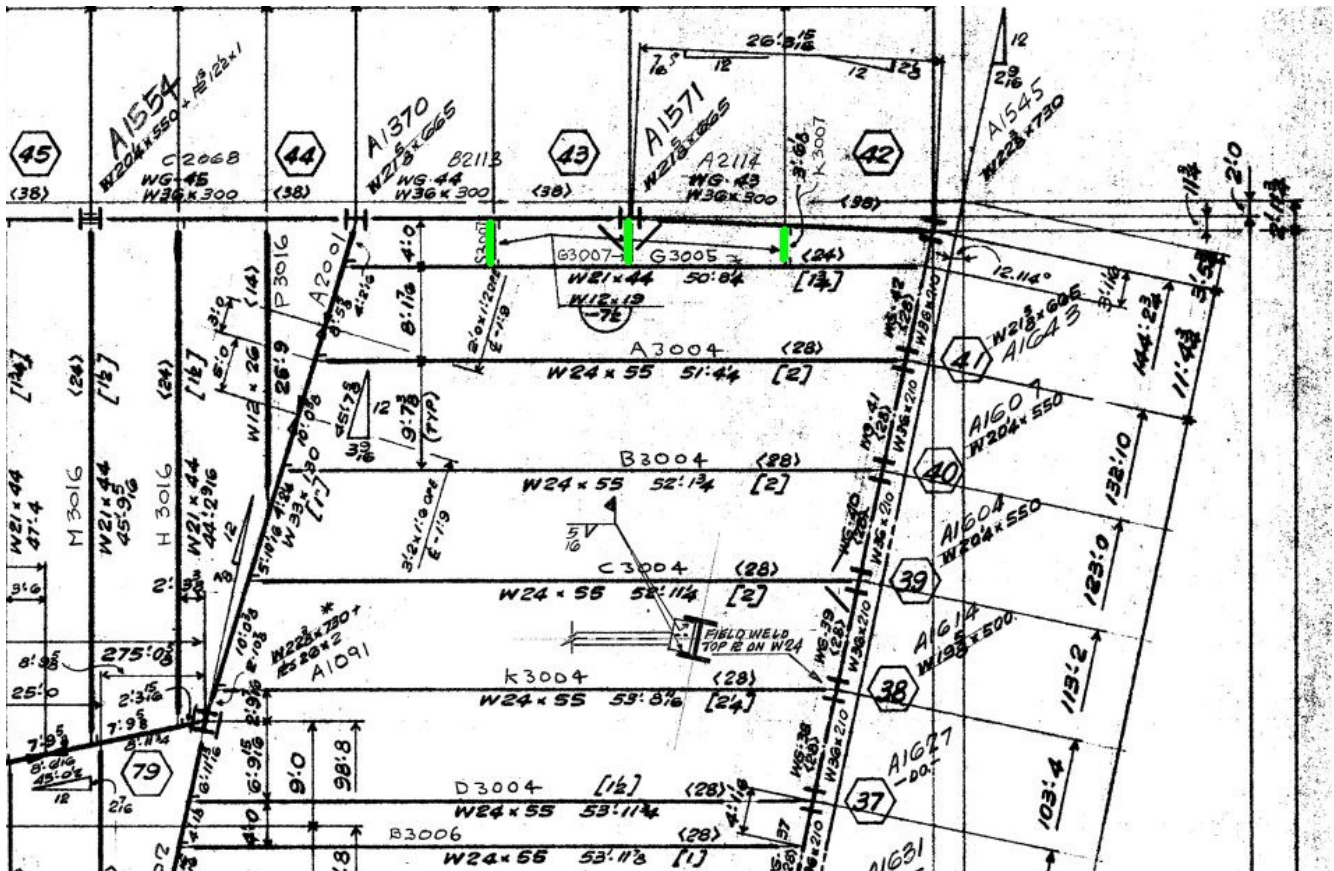
Figure 12: Three W12 x 19 lateral support beams labeled S3007, G3007, and K3007 framing into beam G3005 are shown on Frankel drawing #E12/13 (the three beams are highlighted in green here).
