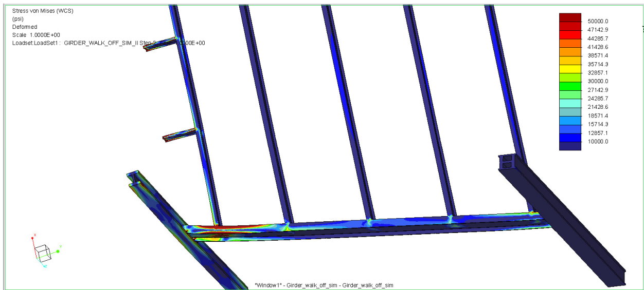
Figure 16: Analysis results showing beam G3005 when it is thermally expanded at 600 °C temperatures and girder A2001 heated to 500 °C temperatures per the NIST WTC 7 report.
