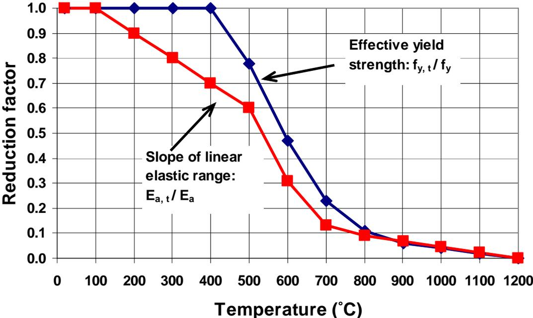
**Figure 9.** Reduction factor for effective yield strength given as ratio of yield strength  $f_{y,t}$  at temperature  $t$  to yield strength  $f_y$  at 20°C, and reduction factor for modulus elasticity given as ratio of slope  $E_{a,t}$  of linear elastic range at temperature  $t$ , and to slope  $E_a$  of linear elastic range at 20°C, per Eurocode 3 (ECFS 2005).
