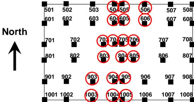
Figure 8. Core columns estimated to be heavily damaged or destroyed in numerical simulation.
