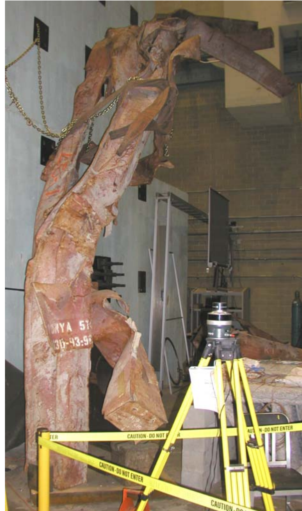
Figure 6–5. WTC 1 exterior panel hit by the nose of the aircraft.
