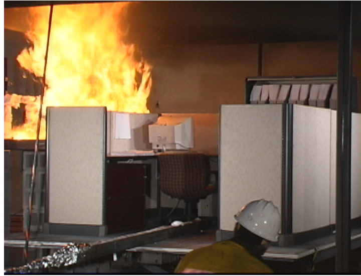
Figure 6–31. Fire test of a single workstation.
