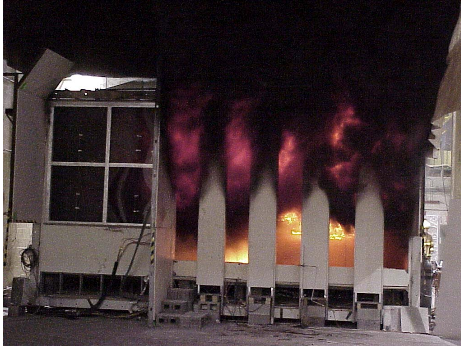
Figure 6–34. Three-workstation fire test, 2 min after the start.
