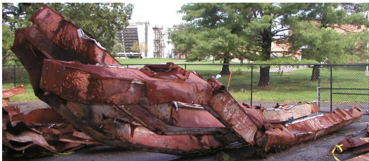
Figure 6–4. WTC 1 exterior panel hit by the fuselage of the aircraft.
